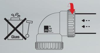
Insert pipe and Tighten cap completely
